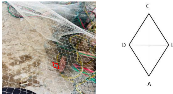
Figure 5. Geometric Shapes of Trawl Nets
